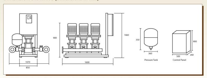
Sample dimension drawing for three pumps system, dimensions to change for other different models. Dimensions above are approximate and subject to final adjustment.
